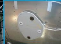
Two patch antennas 2.4 / 1.2 GHz
